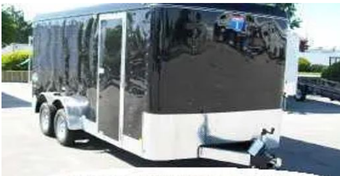
16ft Tandem Axle, 2-3500lb Axles With Ramp
